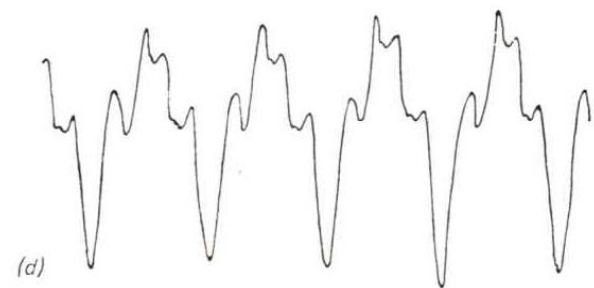
3. 1. The variation in the pressure of the air for a note from (a) flute (b) clarinet, (c) oboe, (d) saxophone.
